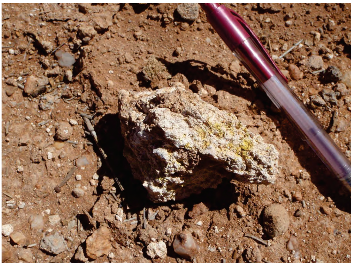
Figure 2: Surface secondary carnotite (uranium) mineralization in calcrete from Baltic Bore
